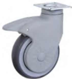
3091 Nylon yoke caster with TPR wheel PP core, ball bearing
